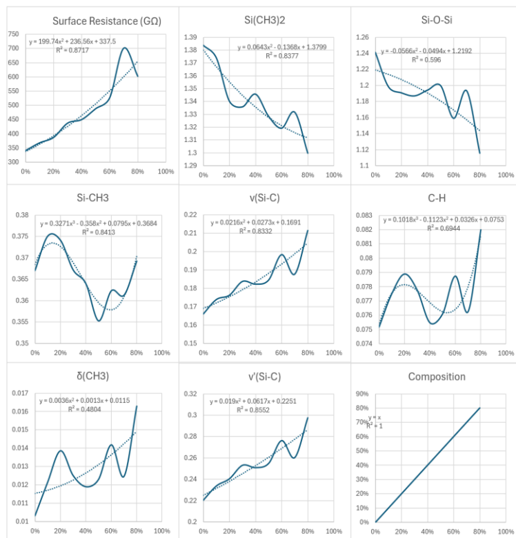
Figure 6 Variable trend analysis for SRF-A: surface resistance ( R_s ) and FTIR-derived predictors across filler loading levels (0–80%).
