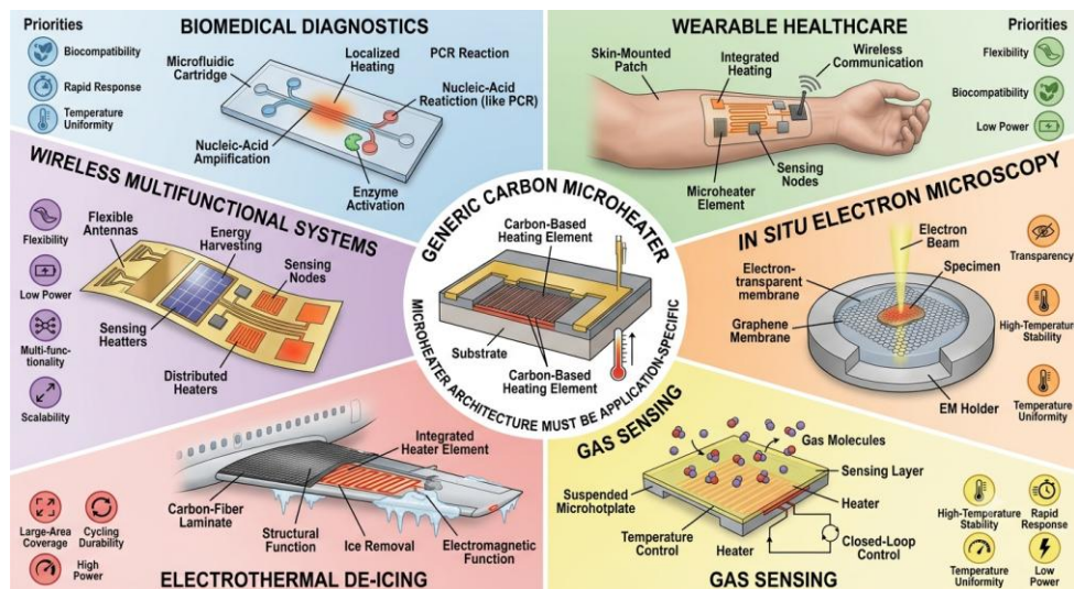
Figure 6 Application ecosystem and design requirements of carbon-based microheaters across biomedical diagnostics, wearable devices, in situ microscopy, gas sensing, structural de-icing, and wireless multifunctional systems. This figure is an author-generated conceptual synthesis of the reviewed literature and should not be interpreted as a quantitative experimental dataset.
