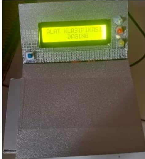
Figure 5 electronic nose for meat classification
