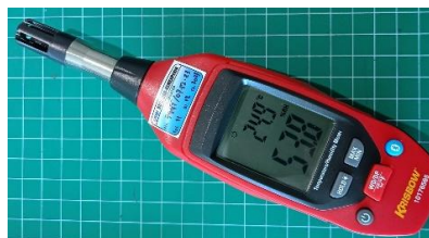
Figure 2. KAN-certified temperature and humidity measuring device
