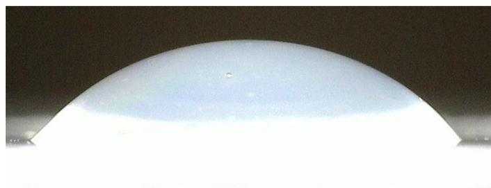
Figure 8 Polypropylene Contact Angle 180 second plasma treatment
