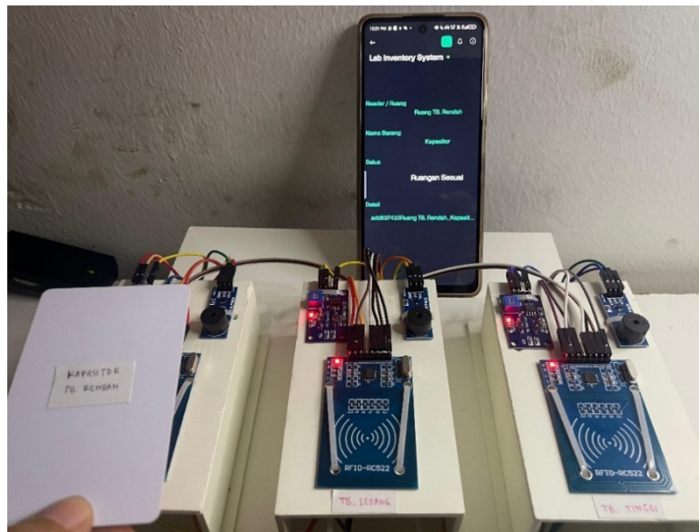
Figure 10. Low-risk material placement test. The capacitor's RFID tag matched the low-hazard compartment and no alarm was raised.
