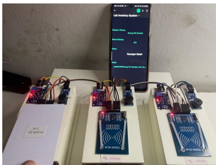
Figure 11. Medium-risk material misplacement test. The system detected the hazard-level mismatch and issued an alarm despite normal environmental readings.
