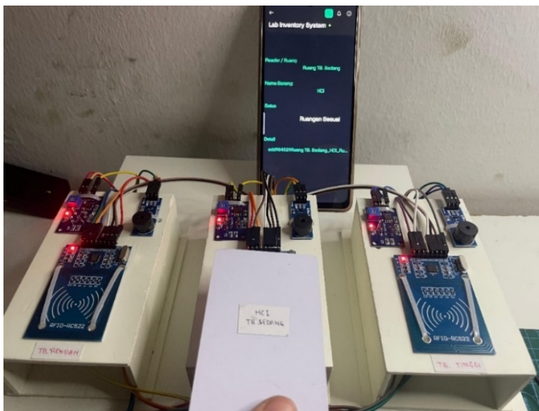
Figure 9. Medium-risk material correct placement test. The HCl tag matched the medium-risk compartment, and no alerts were generated.
