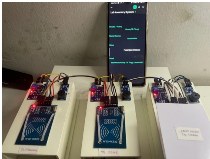
Figure 12. High-risk compartment test. The system flagged the placement of a medium-risk material in a high-risk compartment as non-compliant.
