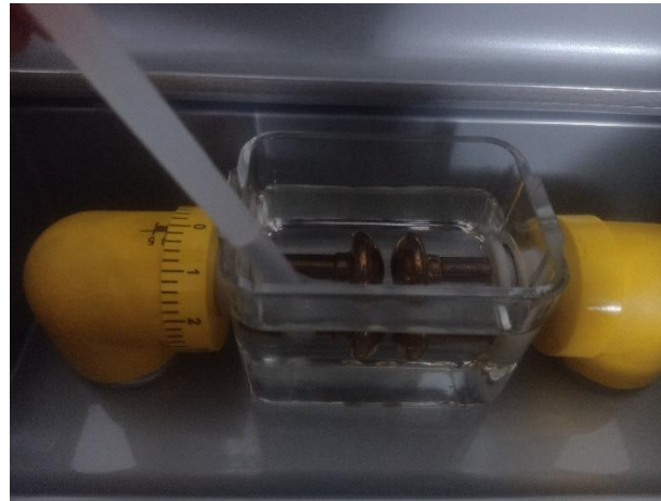
Figure 1 Testing the breakdown voltage value of insulating oil using the IEC Standard BAUR Oil Tester DPA
